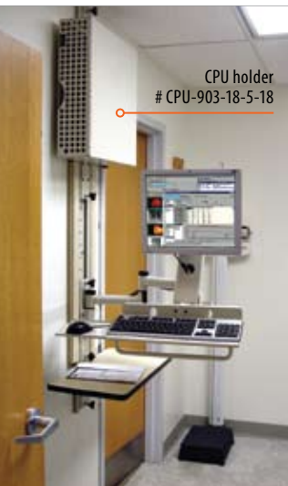
J. Custom Wall Mount with Z-series combo arm, CPU holder, and foldable shelf
