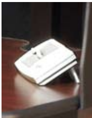
Environmental heating and cooling system controlled at the workstation
