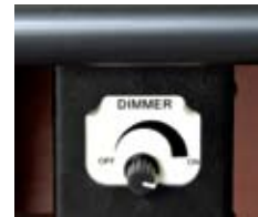
Dimmer switch for LED backlight
